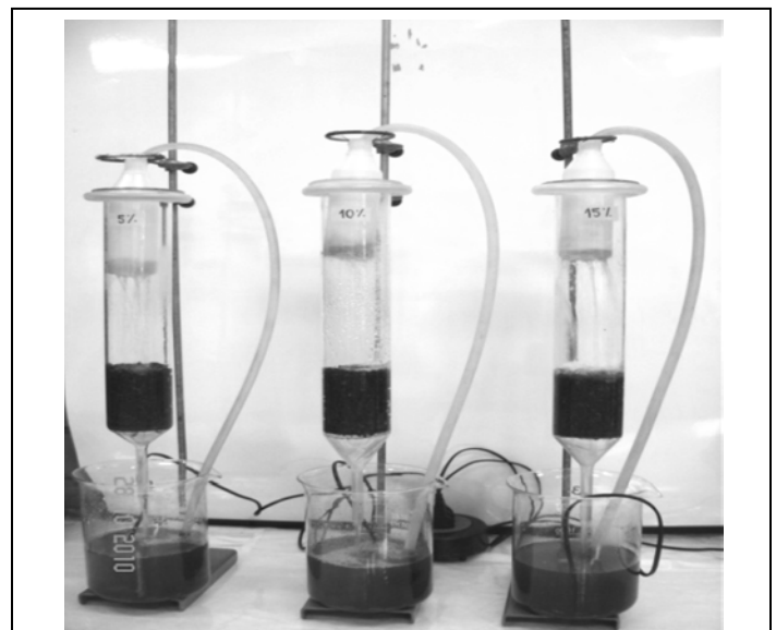
Fig. 2 Glass leaching (recirculating) columns.
